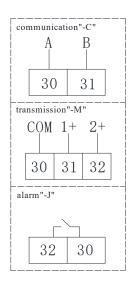
An example of wiring for the communication part is shown below:
